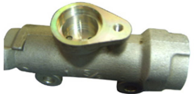
Honda style reservoir bore before installation of Super-Duty Adaptor
